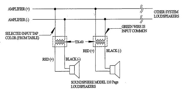
Remember to clip and insulate unused input wires; shorting any input wire to another will reduce the volume level and place an unexpected load on the power amplifier.
